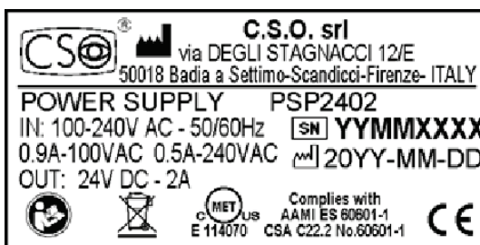
Fig 3 - Power supply PSP2402 data plate
