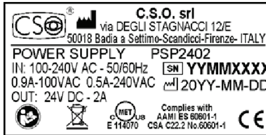
Fig 3 - Power supply PSP2402 data plate
